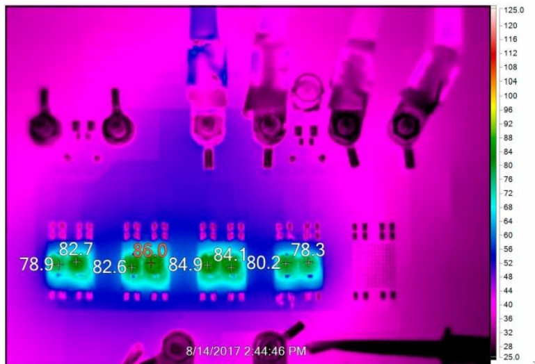
Figure 9. Thermal @ V_{IN} = 12V , V_{OUT} = 1.0V , I_{OUT} = 180A , T_A = 25^\circ C , 400LFM Airflow
